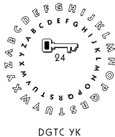
Figure 2-4 Four Caesar cipher keys—1, 2, 24, and 25—encrypting FIVE AM.
