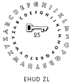
Figure 2-4 Four Caesar cipher keys—1, 2, 24, and 25—encrypting FIVE AM.
